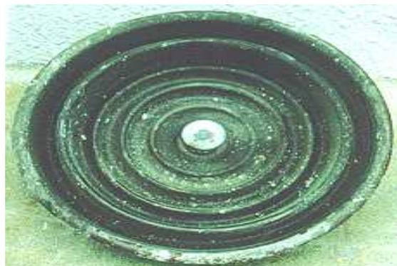
Fig-1: Pollution Deposits On Insulator Strings Due To Industrial Emissions
