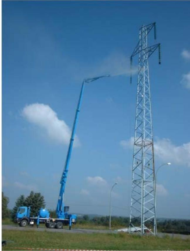
Fig 9 : Telescope Boom Insulator Washer
