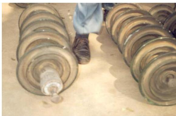
Fig-4: Dust Accumulation On Insulators
