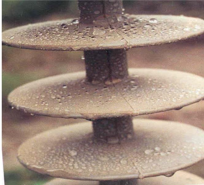
Fig-8 :Hydrophobic Surface of Composite long rod insulator
