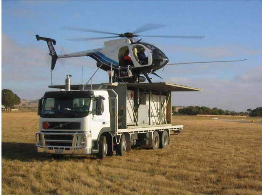
Figure –10: Truck mounted Helipad
