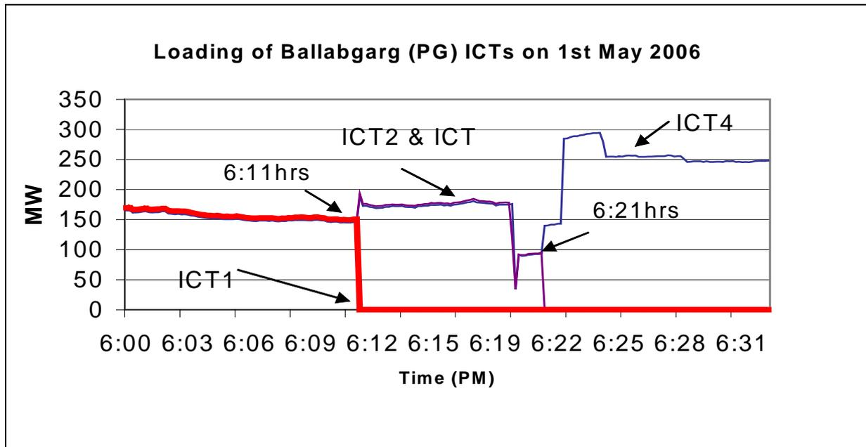
Ballabgarh 400/220 kV substation (POWERGRID) houses four ICTs of 315 MVA each, which were in operation at the time of incident and were equally loaded as shown above. At 18:11:42 hrs ICT- 1 tripped and reportedly caught fire. ICT 2 and 3 were manually tripped at 18:21:10 Hrs as they were adjacent ICT -1, in the proximity of fire. ICT -4 however continued to remain in service.
