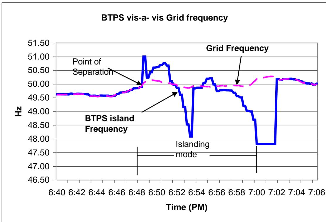
BTPS unit # 3 tripped at 18:19.44.419 Hrs on over voltage, at the time of second fault (Blue phase - earth fault). The output reduced to 455 MW and stabilized at around 550 MW at this point of time till islanding. During islanding, it generated from 500 to 550 MW with varying frequency as shown above.
